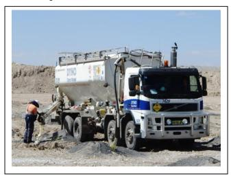
TITAN 9000xero can be delivered through a standard MPU into the blasthole via auger or pump
